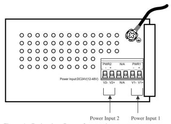
**Figure 8: Redundant Power Connections**
