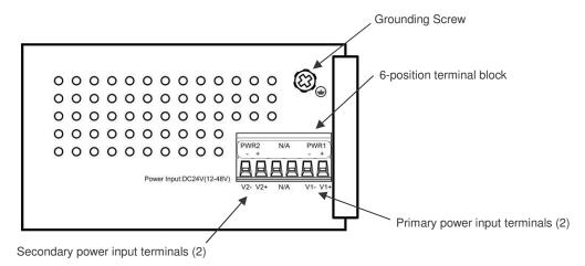
Figure 2: SISTF1010-150-LR(T) Industrial Switch (Bottom View)
