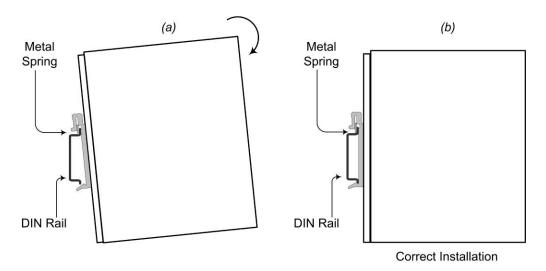
Figure 5: Industrial Switch Mounting to DIN Rail
