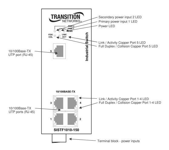
Figure 1: SISTF1010-150-LR(T) Industrial Switch (Front View)
