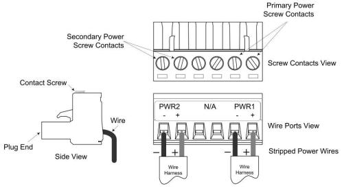
Figure 9: 6-Position Terminal-Block (Primary/Redundant Power Wiring)
