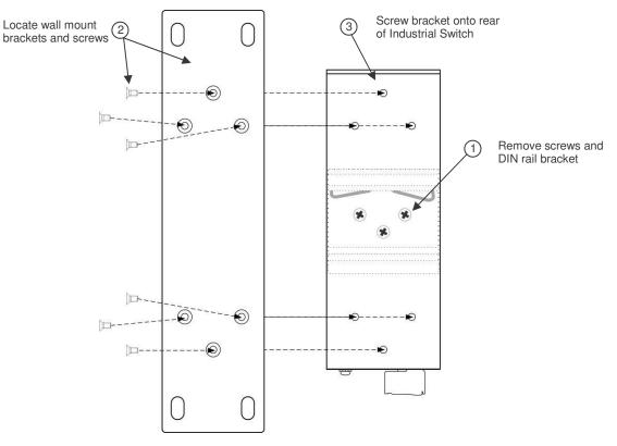
Figure 6: Installing wall mount bracket to Industrial Switch
