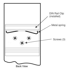
Figure 4: Mounted DIN Rail Clip
