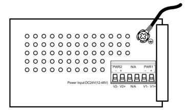
Figure 7: Industrial Switch Ground Screw (Bottom Panel)
