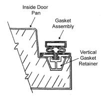
NOTE: The gasket may appear too large, but if it is installed as indicated above it will slip into place.
