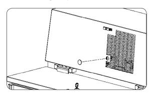
The temperature control is located behind the silver plug on the front side of the system area (dial thermometer side). To adjust, remove the plug turn the adjustment screw with a pair of pliers a small amount at a time; turning clockwise lowers the temperature. An "OFF" position is fully counterclockwise and interrupts power to the compressor and condenser fan only, not the entire refrigerator.
