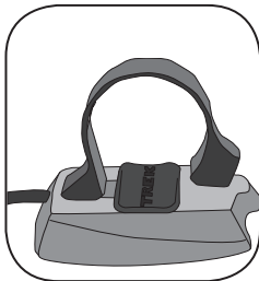
Figure 4- Clamp and friction pad in computer base
