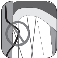
Figure 2- Keep the wire out of the spokes
