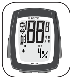
Figure 15- Set Units screen items (which show up one at a time during set-up)
