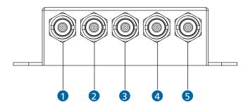
RED BNC VIDEO OUTPUT: Connect the Red output to the Red input of the HXMINI5 Receiver using a 75 Ohm coax cable
