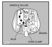
The wire coloured green and yellow must be connected to the terminal marked with the letter  $\times E$  or by the earth symbol  $\frac{1}{2}$  or coloured green and yellow.
