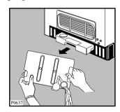
The reservoir must be re-inserted correctly.
