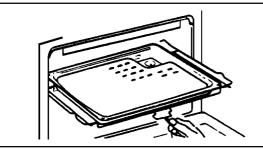
• Adjust the grid and grill pan runner position to allow for different heights of food.
