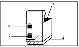
To move the cooker, open the main oven door and lift the cooker by holding inside the top of the compartment.
