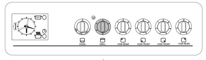
• Turn the grill control to the required setting. The highest number represents the hottest setting and the lowest the coolest setting.
