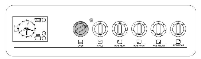
• To operate the oven simply set the oven control dial to the required temperature.
