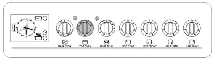
• Turn the top oven temperature control to the required setting.
