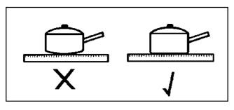
The size of the base of the saucepan should be the same or up to 2.5cm/1inch larger than the hotplate. If the base is too small, energy will be wasted, boilovers will also be more difficult to deal with as spillage will fall directly onto the hotplate.
