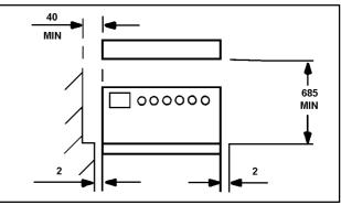
It is important to ensure that the appliance is level after installation. Levelling feet are fitted to the front of the appliance to accommodate uneven floors.
