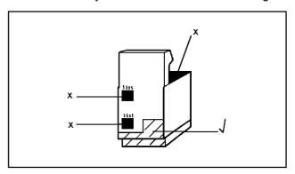
Side walls which are above hob level should be protected by heat resistant non-combustible material and MUST NOT be nearer than 40mm to the hob side.
