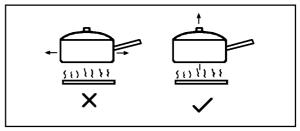
Avoid placing fish kettles or large preserving pans across two hotplates as this may cause damage.
