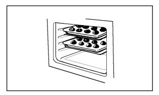
Do not line any part of the oven with foil as it may cause damage or interfere with the air circulation.
