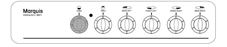
• To operate the oven turn the oven control to the required temperature.
