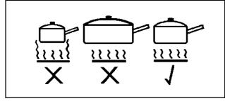
**Pressure cookers, preserving pans** etc., should comply with the recommendations given above. Traditional round bottomed Woks **must not be** used even with a stand. Woks with flat-bottomed bases are available and do comply with the above recommendations.
