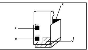
To move the appliance, open the oven door, and lift the appliance by holding inside the top of the oven compartment.
