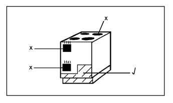
To move the appliance, open the main oven door, and lift the appliance by holding inside the top of the compartment.
