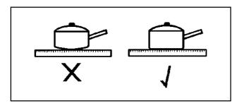
The size of the base of the saucepan should be the same or up to 2.5cm/1 inch larger than the hotplate. If the base is too small, energy will be wasted, boilovers will also be more difficult to deal with as spillage will fall directly onto the hotplate.
