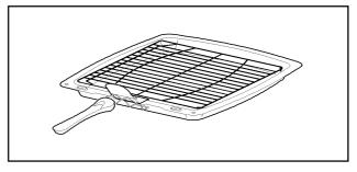
To remove the handle, slide the handle to the right and lift the handle away from the cut out on the grill pan.
