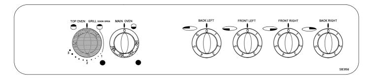
Turn the top oven temperature control to the required setting. Our diagram shows the oven set to 150°C. Close the oven door.
