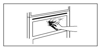
DO NOT ATTEMPT TO REMOVE ANY OF THE CONTROL KNOBS FROM THE APPLIANCE AS THIS MAY CAUSE DAMAGE AND IS A SAFETY HAZARD.
