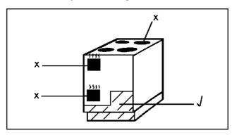
To move the appliance, open the main oven door, and lift the appliance by holding inside the top of the compartment.
