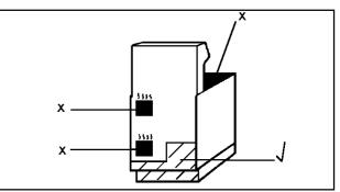
To move the appliance, open the main oven door, and lift the appliance by holding inside the top of the oven compartment.
