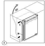
Screw appliance into place and retain the cabinet with screws (I) through the securing brackets into the worktop or adjacent woodwork as necessary.
