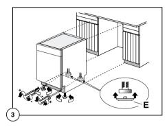
If necessary, pads (E) are supplied for the rear feet to make sliding the appliance in and out of the recess easier. To fit the pads, press them onto the rear feet. If required, the dimensions of these pads can be reduced by breaking them where marked.
