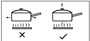
Avoid placing fish kettles or large preserving pans across two hotplates as this may cause damage.
