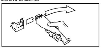
To correctly locate the grill pan ensure the pan locates into the runners in the grill compartment side panels. There are two alternative positions.
