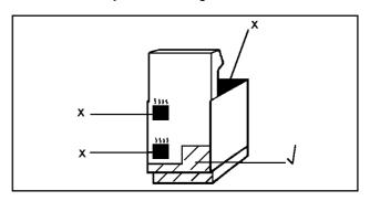
To move the appliance, open the oven door, and lift the appliance by holding inside the top of the oven compartment.
