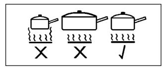
The saucepan base should cover the hotplate as much as possible. A base diameter of up to 225mm (9") may be used on a 180mm (7") hotplate.
