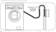
Firstly form a hook in the end of the drain hose using the «U» piece supplied. Place the drain hose into your standpipe, which should have an internal diameter of approximately 38mm thus ensuring there is an air break between the drain hose and standpipe. When discharging into a standpipe ensure that the top of the standpipe is no more than 90 cm (35.4") and no less than 60 cm (23.6") above floor level.
