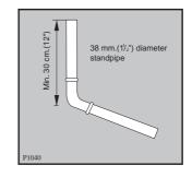
Make sure that it is designed in such a way, that the end of the drain hose cannot be covered with water.
