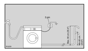
Make sure that it is designed in such a way, that the end of the drain hose cannot be covered with water.
