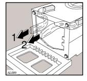
Place the machine in an upright position and remove the three plastic spacers.
