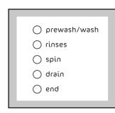
After the machine has started, only the running phase pilot light stays on.
