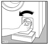
Unscrew and remove the filter.
