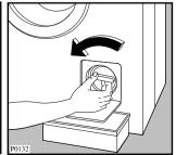
Unscrew and remove the filter.
