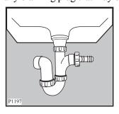
Push the drain hose onto the spigot and secure with a clip, ensure a loop is formed in the drain hose (see diagram) to prevent waste from the sink entering the washing machine.
