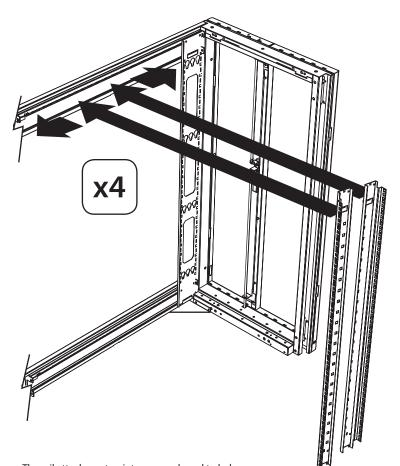
The rail attachment points are numbered to help you align each pair of rails at the same depth. Before attaching the rails using the screws (shown in Step 6-3), make sure the same number appears in all three windows. **Note:**Number shown in Step 6-2 is for illustration purposes only; attach rails at desired depth.
