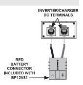
Securely tighten the Inverter/Charger's DC terminals to prevent the red battery connector's wires from coming loose due to accidental stress or tension.
