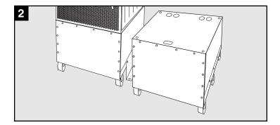
Using the included bolts, install one mounting bracket on each side of the battery module compartment, as shown. If desired, install the bracket to the floor surface with user-supplied hardware. If the mounting brackets are not attached to the floor, ensure the rear caster wheels are locked to prevent the SUBF2030 from rolling and causing a potential hazard.
