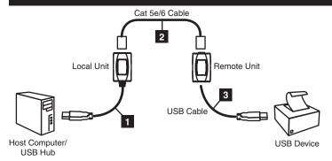
Note: Diagram shows the B202-150. Connections will be the same for the B202-150-WP, except separate USB A/B device cables will be needed.
