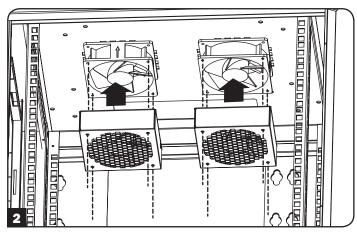
2 Mount the shroud casing over the fans using the supplied hardware.
