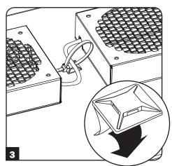
**3** Secure the wire between each fan to the cabinet using the peel-and-stick cable anchor with tie.
