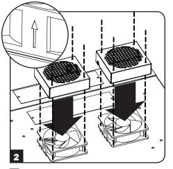
2 Mount the assembly over the vents on the exterior of the Wall-Mount cabinet, threading the screws from the inside of the cabinet.
