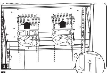
Mount the SRFANWM over the vents inside the Wall-Mount cabinet using the supplied hardware, with airflow arrows and label facing toward the top of the cabinet.
