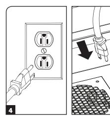
Plug the SRFANWM input cable into a power source, such as an external source. For connection to an internal PDU, utilize the removable cable access panel.
