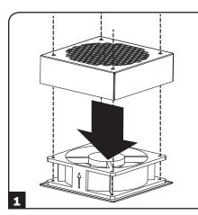
**1** For external installation, begin by installing the fan into the shroud using the supplied hardware.
