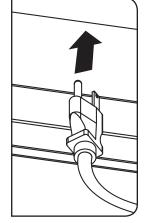
Plug the SRFANWM input cable into a power source, such as an internal PDU. For external power connection, utilize the removable cable access panel.
