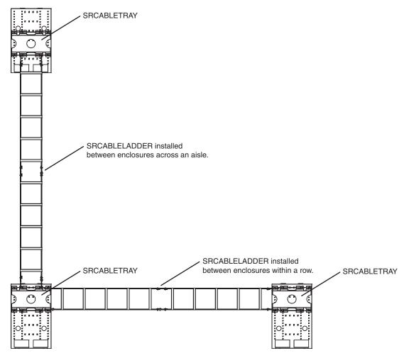
Use a tape measure to determine the distance that SRCABLELADDER will bridge. (Preassembling the ladder sections will allow you to observe their attachment points in place for a more accurate measurement.)
