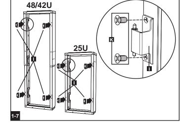
1-7 Use two M6 x 12 mm flat-head screws K to attach each hinge
