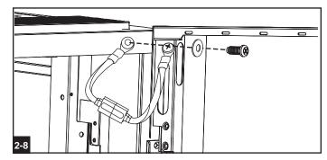
**2-6** Use two M6 x 12 mm screws and washers **L** to connect the included grounding cable **N** from the rack enclosure to the extension frame.
