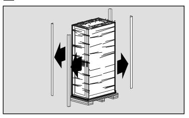
Remove two brackets attaching enclosure to pallet. Save brackets to either permanently mount enclosure to floor in final installation or for use in repacking the enclosure.
