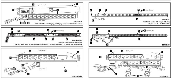
Digital Load Meter BMultiple High-Quality Outlets CLong Input Cord with High Quality Input Plug AC Circuit Breaker Protection Secure Mounting Hardware Rugged All-Metal Housing Grounding Lug Twist-Lock L5-20P to Straight-Blade 5-20P Plug Adapter Dual Circuits JLighted Power Switch with Safety Cover Cord Retention Bracket
