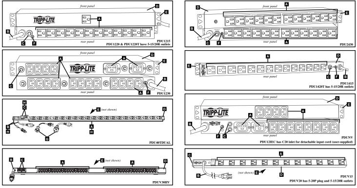
Multiple High-Quality Outlets Long Input Cord with High-Quality Input Plug AC Circuit Breaker Protection Rugged All-Metal Housing Escure Mounting Hardware Grounding Lug Twist-Lock L5-20P to Straight-Blade 5-20P Plug Adapters Dual Circuits
