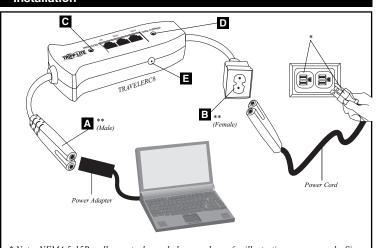
\* Note: NEMA 5-15R wall receptacles and plug are shown for illustration purposes only. Since the power cord is user-supplied, wall receptacle and plug style will vary depending on the user. Both Traveler In-Line models are compatible with worldwide voltages (automatically switching between 120V and 240V).
