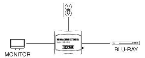
1 Connect the longer HDMI cable between the source and the INPUT port on the B122-000-60.
