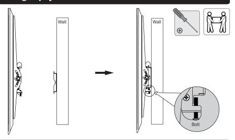
Tighten the two bolts by using an appropriate phillips screwdriver to secure bracket.
