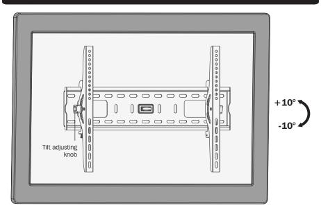
Loosen the adjusting knobs to tilt to desired angle then retighten the knobs.
