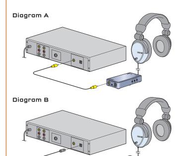
Connecting the AX360 to a DVD player or audio receiver is easily achieved through either the digital optic or coaxial port. Diagram A shows connecting via the digital coaxial. Diagram B shows connecting via the digital optic port. The AX360 audio controller has is a selector switch that must be positioned to either optic or coaxial depending on which connection you use.
