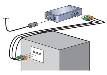
The AX360 audio controller includes analog 5.1 outputs. Through these outputs you can connect to a 5.1 speaker system that is "self-powered", meaning that the speaker system has its own amplification. Connect the speakers accordingly per the description:
