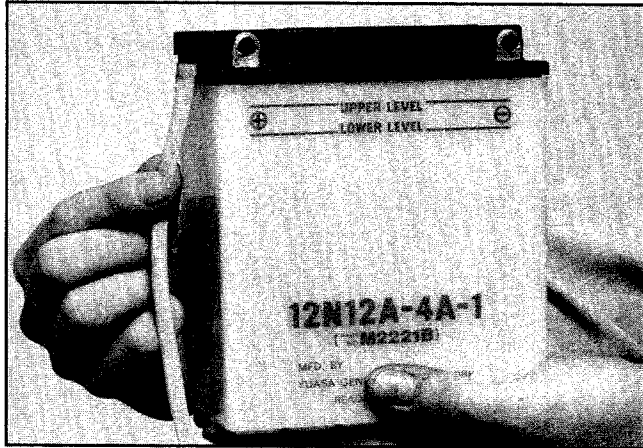
Photo 2-24: Attach vent tube to battery.
