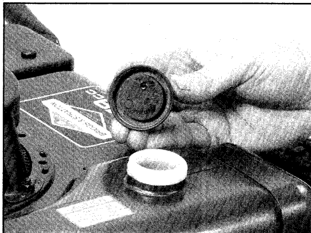
Photo 4-2: Fuel tank on 8HP engine (24" mower).
