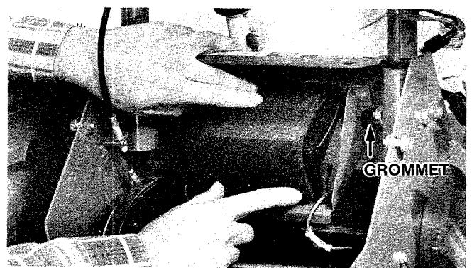
Photo 5-53: Installing the battery.
