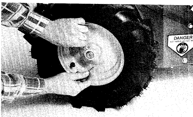
Photo 5-8: Removing the wheel.
