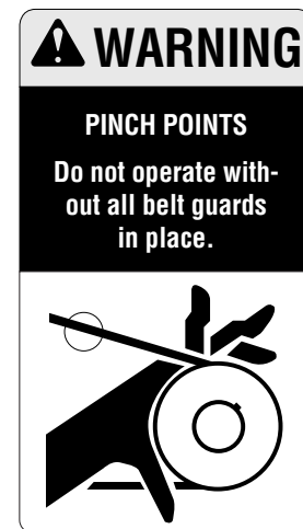
Beneath belt/pulley cover
