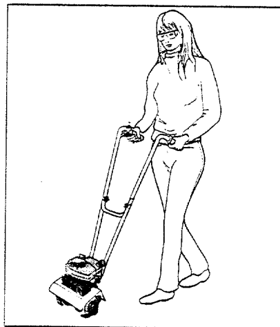
Figure 11: Operating position. Do not use engine throttle lever unless you are in this position.
