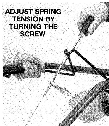
Photo 5-14A: Adjusting the length of the Clutch Bail Spring.
