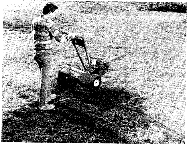
Photo 4-2: When you reach the end of a row, slow the engine down and lift up on the handlebars to raise the tines from the soil.
