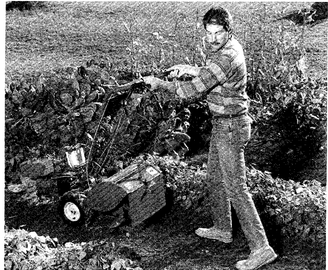
Photo 4-17: To turn around in cramped quarters, move close to obstacle, then put the tiller in Reverse while lifting up on the handlebars (to raise the tines out of the soil) and turning the tiller.
