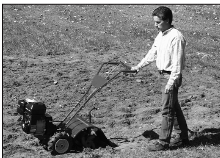
Fig. 4-2: Use one hand to guide tiller when moving forward.
