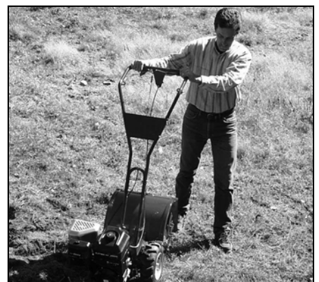
Fig. 4-5: With tines out of ground, push handlebars sideways to turn tiller.
