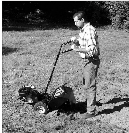
Figure 4-4: To begin turn, lift handlebars until engine and tines are balanced over wheels. Be sure tines are out of ground.
