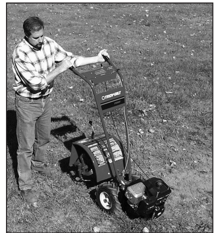
Figure 4-5: With tiller balanced over wheels (and tines out of the ground), push handlebars sideways to turn tiller.
