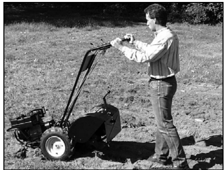
Figure 4-4: Find balance point before turning.
