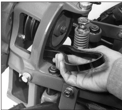
Figure 5-20: Shift into FORWARD and remove the belt.
