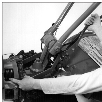
Figure 4-12: High range to low range. Shows moving belt from top-front groove onto top-rear pulley groove.
