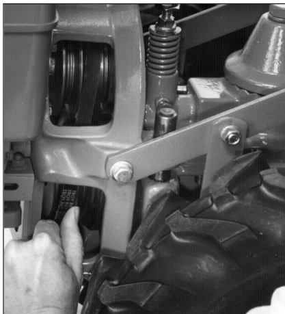
Figure 4-10: Low range to high range. Shows moving belt from lower-rear groove onto lower-front groove.
