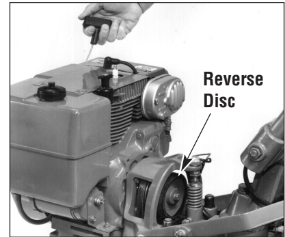
Figure 5-25: Checking Reverse Disc in NEUTRAL.
