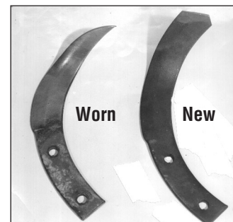
Figure 5-30: Check for wear every 30 operating hours.
