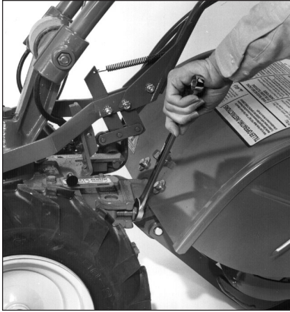
Figure 4-24: Loosening attachment swing-bolts.
