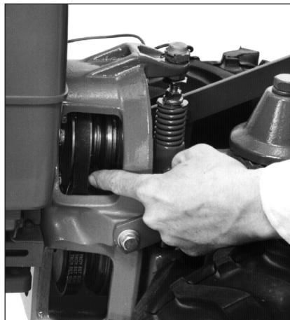
Figure 4-11: Low range to high range. Shows moving belt from top-rear groove onto top-front groove.
