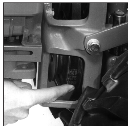
Figure 4-13: High range to low range. Shows moving belt from lower-front onto lower-rear groove.
