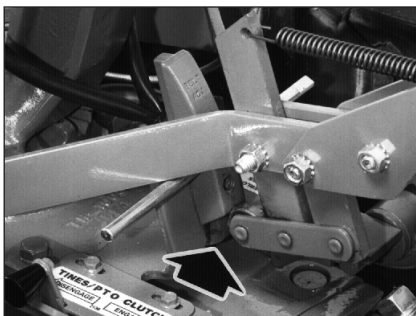
Figure 5-15: With Drive Lever in FORWARD position, clutch roller should be engaged slightly beneath the adjustment block.
