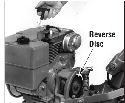
Figure 5-25: Checking Reverse Disc in NEUTRAL.
