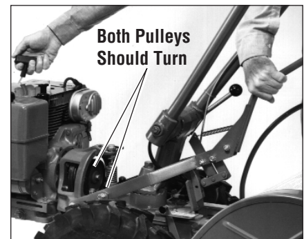
Figure 5-26: Checking Reverse Disc in REVERSE.
